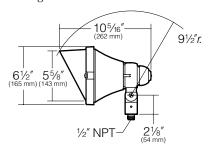
**Housing:** Die-cast aluminum body and lens frame.
