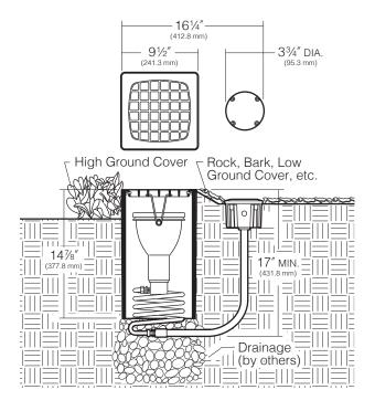
**Housing:** Spun copper, bronze clamping ring, prewired cord through brass seal.
