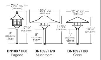
**ORDERING INFORMATION Fixture** Source **Finish** I BN189/3L3KUV¹/NB 5.2W, 3 LED's, 3000K Brass/ Natural I BN189/3L4KUV¹/NB 5.2W, 3 LED's, 4200K IBN189/3L5KUV<sup>1</sup>/NB 5.2W, 3 LED's, 5100K I BN189/3L3KUV¹/VG 5.2W, 3 LED's, 3000K Brass/ Verde I BN189/3L4KUV¹/VG 5.2W, 3 LED's, 4200K
