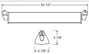
Alternate TEK/HTEK Trac Adapter Compatible with either Juno TEK or HTEK trac systems • System specific and assembled to trac fixture • Integrally polarized construction to prevent reverse installation – only allows insertion in proper orientation • Rotary circuit selector enables simple switching between circuits • Integral on/off switch enables individual fixtures to be switched for servicing.
