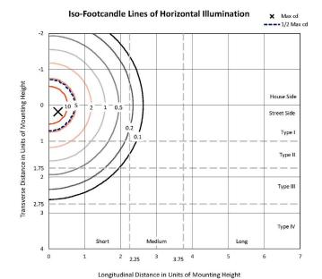
Based on 10 foot mounting height. Maximum calculated value = 18.2 fc
