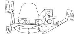
4" Standard ICA Housing 750 lm (11.8W) w/ELK19 Series Module 950 lm (11.8W) w/ELK21 Series Module New Construction
