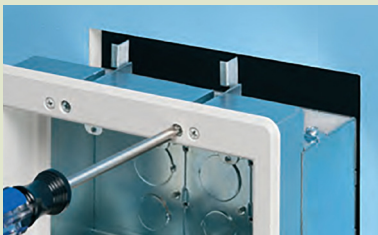
Cut a hole using enclosure without trim plate, as template. Mounting wings hold box in wall.
