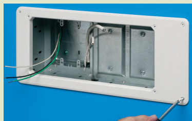
After drywall is installed, add trim plate, then install enclosure assembly to wall with outer screws.
