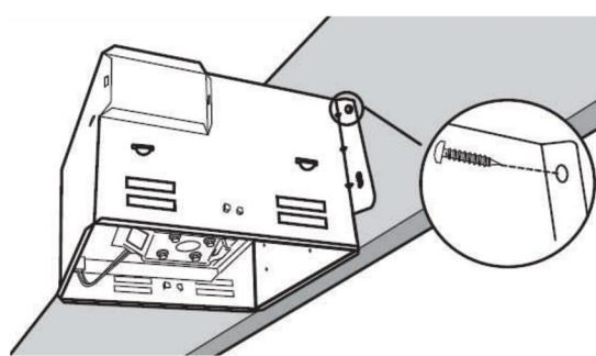
**HOUSING CAN BE INSTALLED USING THE UNIVERSAL MOUNTING BRACKET WITHOUT THE USE OF BAR HANGERS.**
