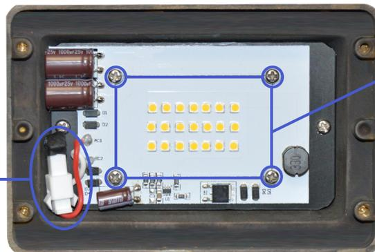
REMOVE THESE 4 SCREWS TO RELEASE THE LED BOARD
