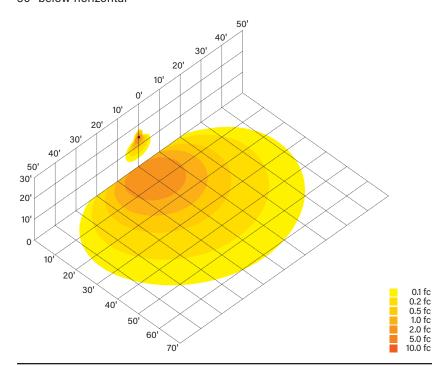
Ground mounted at 6" above ground, 10° above horizontal, shining towards building exterior wall at 14' away
