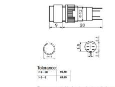
Recommended hole size for installation: Ø12mm
