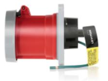
UPC Code : 078477901564 Country Of Origin : Mexico 60 Amp, 277/480 Volt 3-Phase, 4P, 5W, LEV Series North American-Rated IEC 60309-1 & 60309-2 Pin & Sleeve Receptacle, Industrial Grade, IP66/IP67/IP68/IP69K, Watertight - Red
