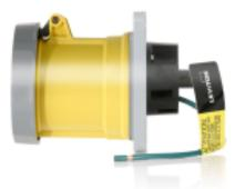
UPC Code : 078477901953 Country Of Origin : Mexico 60 Amp, 125 Volt, 2P, 3W, LEV Series North American-Rated IEC 60309-1 & 60309-2 Pin & Sleeve Receptacle, Industrial Grade, IP66/IP67/IP68/IP69K, Watertight - Yellow
